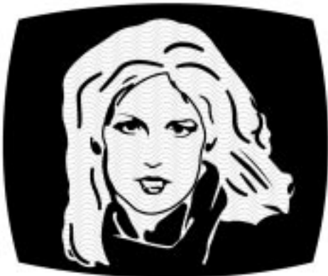
Fig. 11-5. A herringbone pattern caused by adjacent channel interference.
