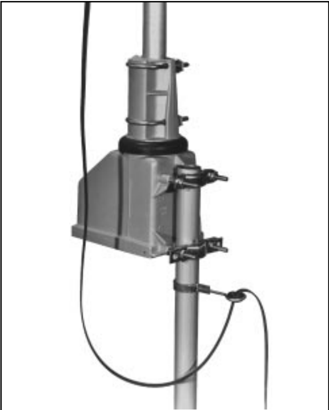
Fig. 8-7. A loop of extra transmission line must be left between the antenna and the drive unit to prevent the line from tangling in the antenna or otherwise restricting its rotation.
